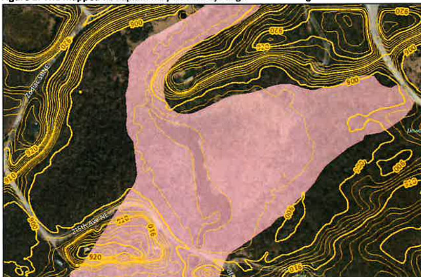
Figure 1: The mapped floodplain may not always align with on-the-ground contour elevations
